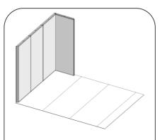
3. Continue erecting walls and aim to place the first roof panel.
