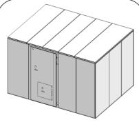
10. Finally, install the last roof panel.
