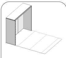
4. Attaching the roof panel will stiffen the structure significantly.
